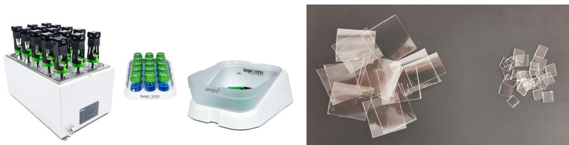
Figure 1. AMPTS system for biogas potential evaluation and PLA cups cut into 1 cm and 0.5cm (mechanical pre-treatment) before addition to AD reactors.
