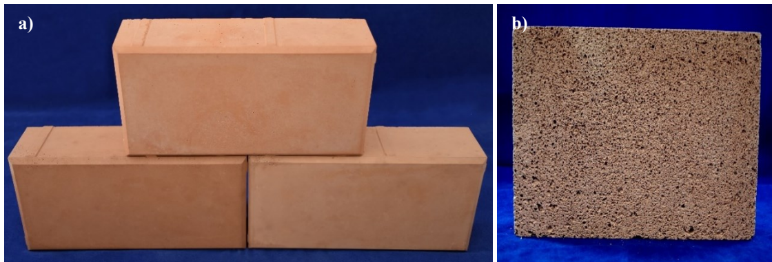
Figure 1. Geopolymer building materials based on brick residues: a) brick, b) lightweight block.
