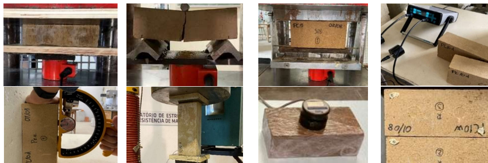
Figure 1 – Mechanical characterization of CEB (from top left to bottom right): compressive strength; flexural strength; splitting tensile strength; ultrasound pulse velocity; pendulum sclerometer; elasticity modulus; shrinkage; thermal conductivity.
