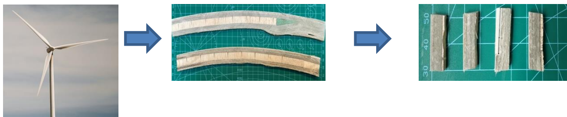
Figure 1. GRP from EoL turbine blades for OL process
