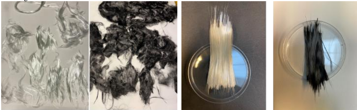
Figure 4. CF (first 2 pics from left side) and GF composite samples
