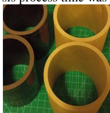
Figure 2. CF (left) and GF (right) composite samples
