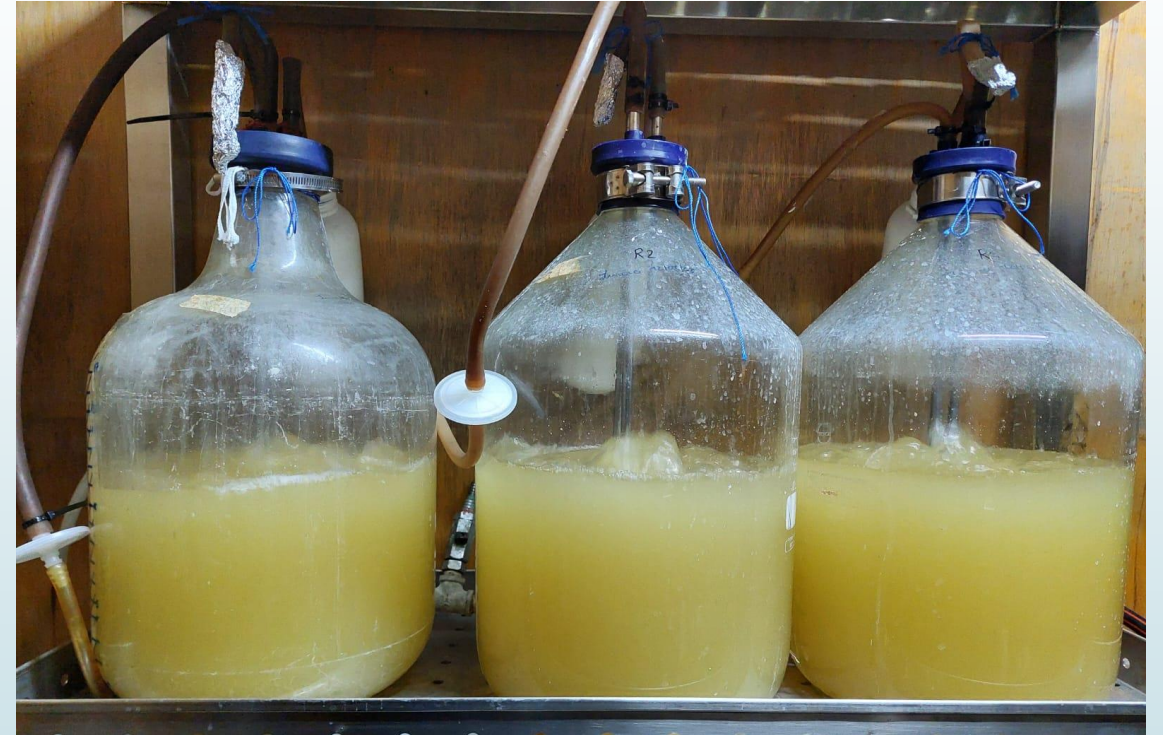
Photograph 2. End of fermentation in Pilot Reactors R1-R2-R3. (72 hours)
