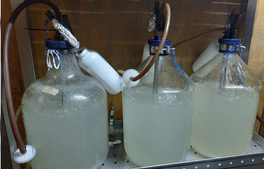
Photograph 1. Start of fermentation in Pilot Reactors R1-R2-R3. (0 hours)
