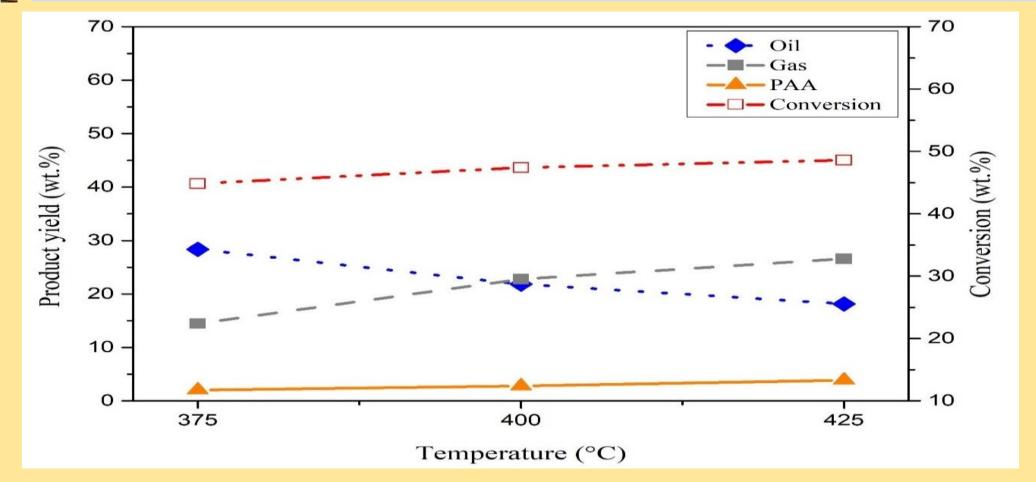
• EWP+HAC co-liquefaction gave maximum oil yield of **28.37** wt.% during co-liquefaction at 375°C
