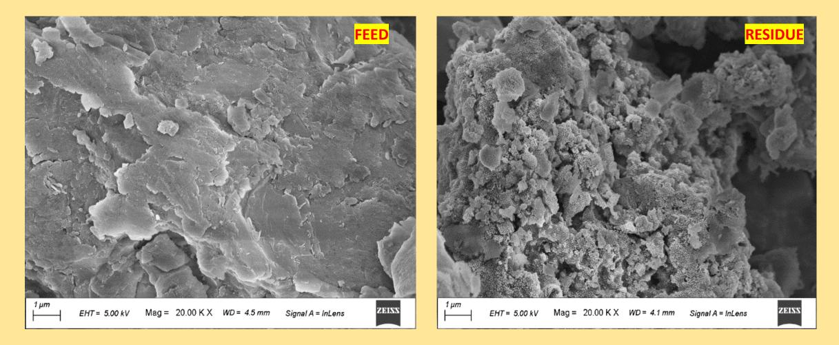
• **Disruption in the residue structure** as well as highly **increased pores** indicate thermal degradation and volatilization of feed samples
