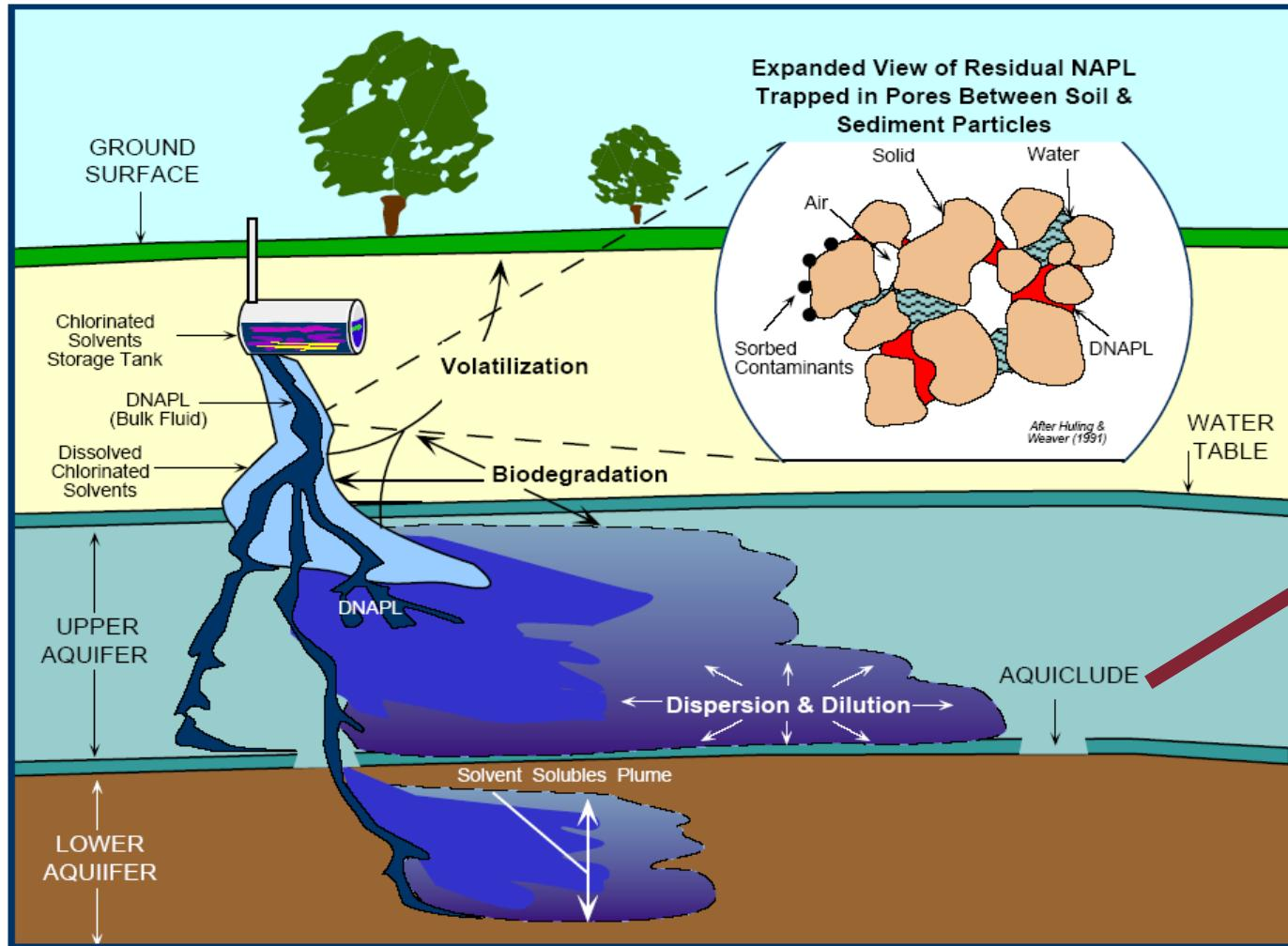
Due to higher density than water, DNAPLs migrates vertically also in the saturated zone (aquifer). Depending on the soil heterogeneity and spilled amount, contamination could reach significant depth.
