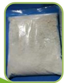
Chitosan obtained from chitin extracted from BSF
