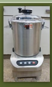
15 min milling and homogenization per 15kg of fresh biowaste
