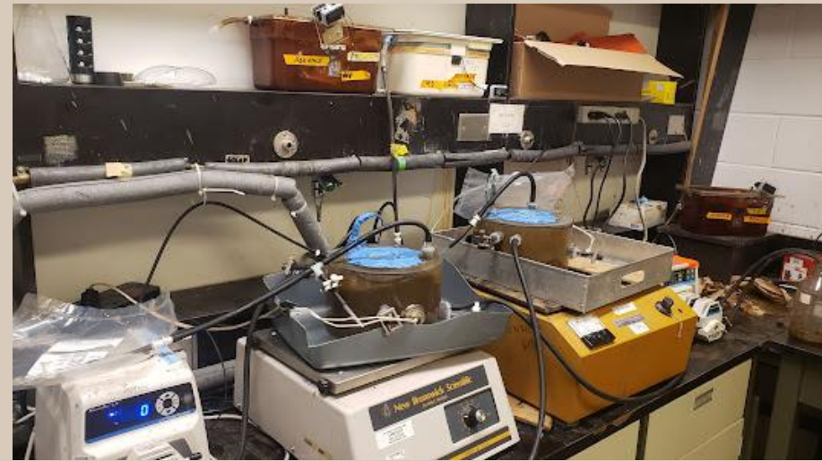
5 L semi-continuous hydrolysis reactors 10 L working volume
