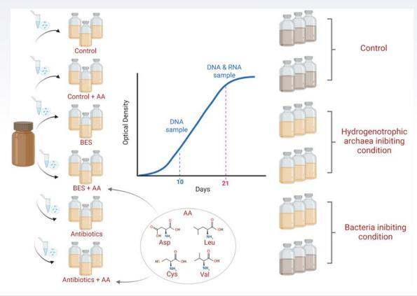
Plan of experimental setup to verify key metabolites involved in the methanation
