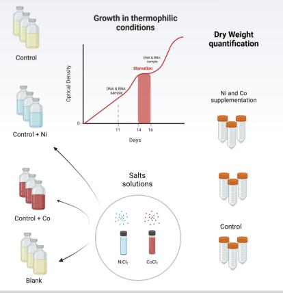
Plan of experimental setup to verify micronutrients involved in the methanation in standard feeding conditions and during H<sub>2</sub> and CO<sub>2</sub> starvation
