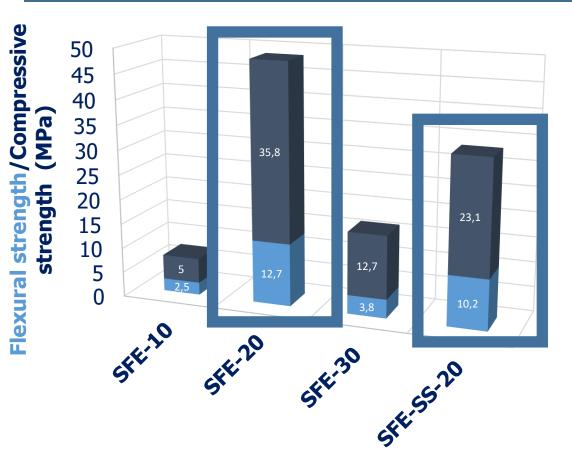
The mechanical properties of the geopolymers using the ASA are superior to those obtained for the commercial activator.
