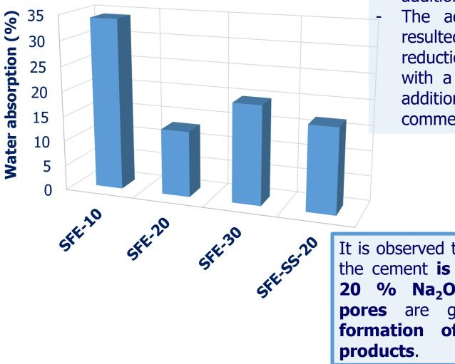
WA is very high with the addition of 10 %  $Na_2O$ . The addition of 20 %  $Na_2O$  resulted in a significant reduction of WA up to 13 %, with a slight increase with the addition of 30 % and when commercial activator is used
