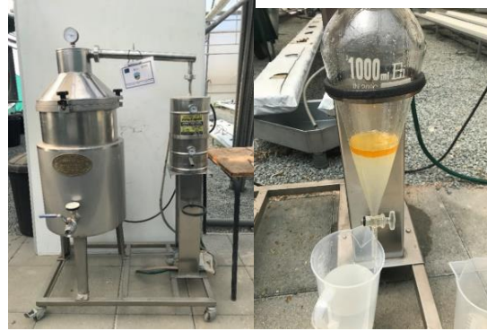
Subjected to hydro-steam distillation for EO extraction
