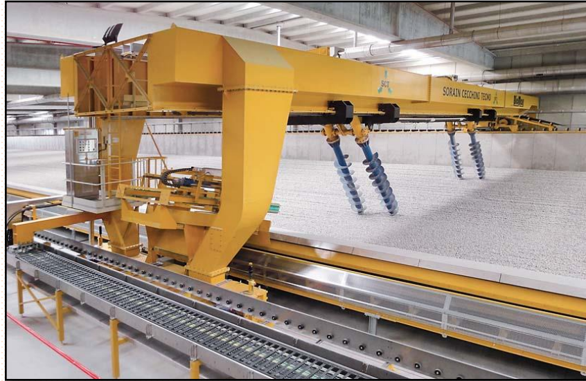
Dynamic windrow process (e.g. Biomax-G®)
