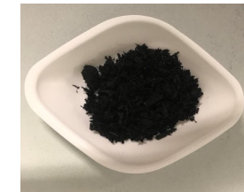
Biochar from KOH-pre-treated digestate
