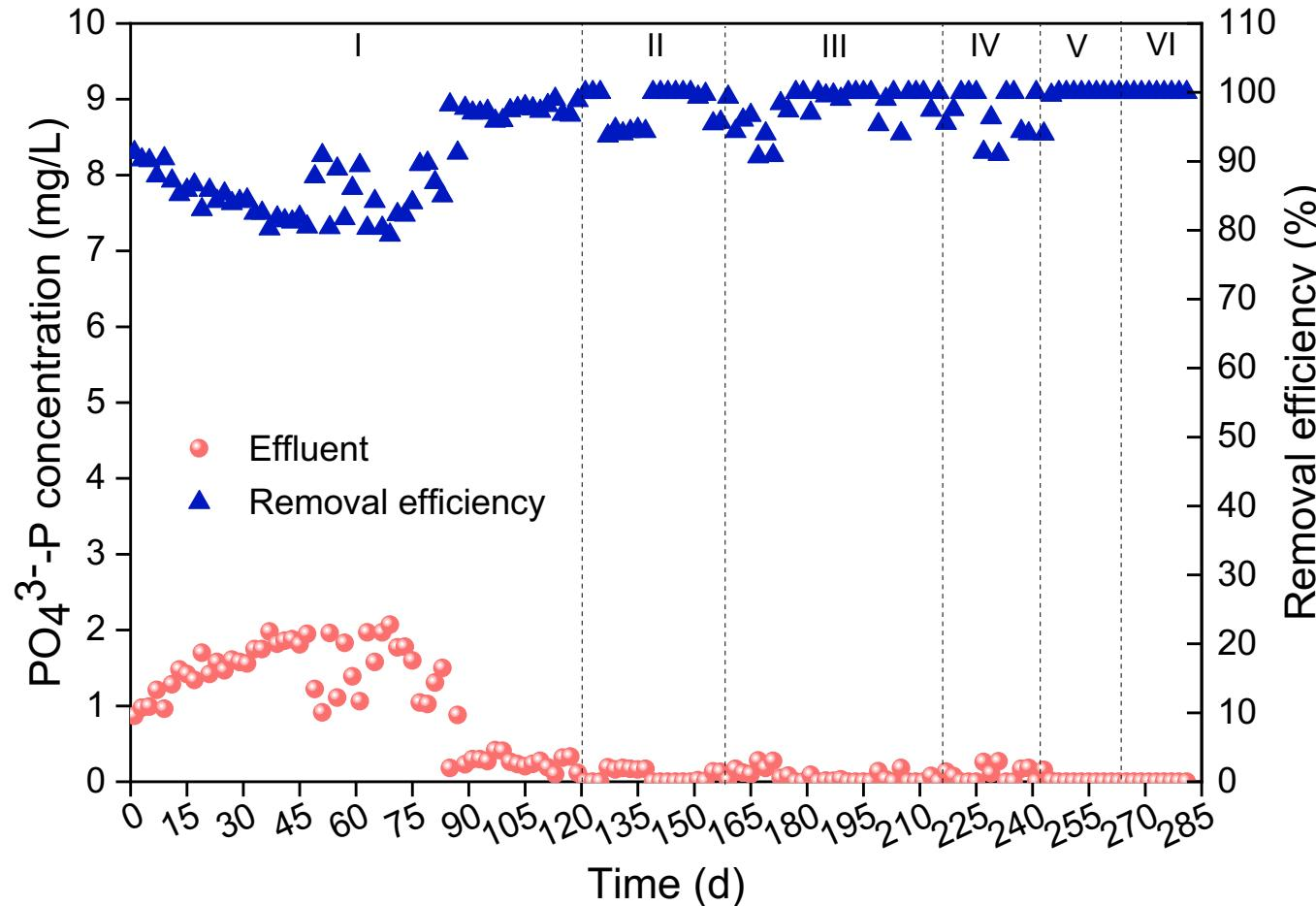
Effluent P concentrations < 0.05 mg/L, when influent P was 3 mg/L.
