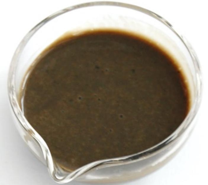
thickened excess activated sludge
