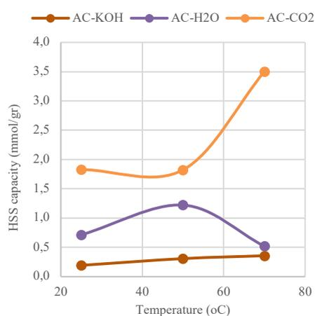
Figure 3. H<sub>2</sub>S capacity of the activated carbons
