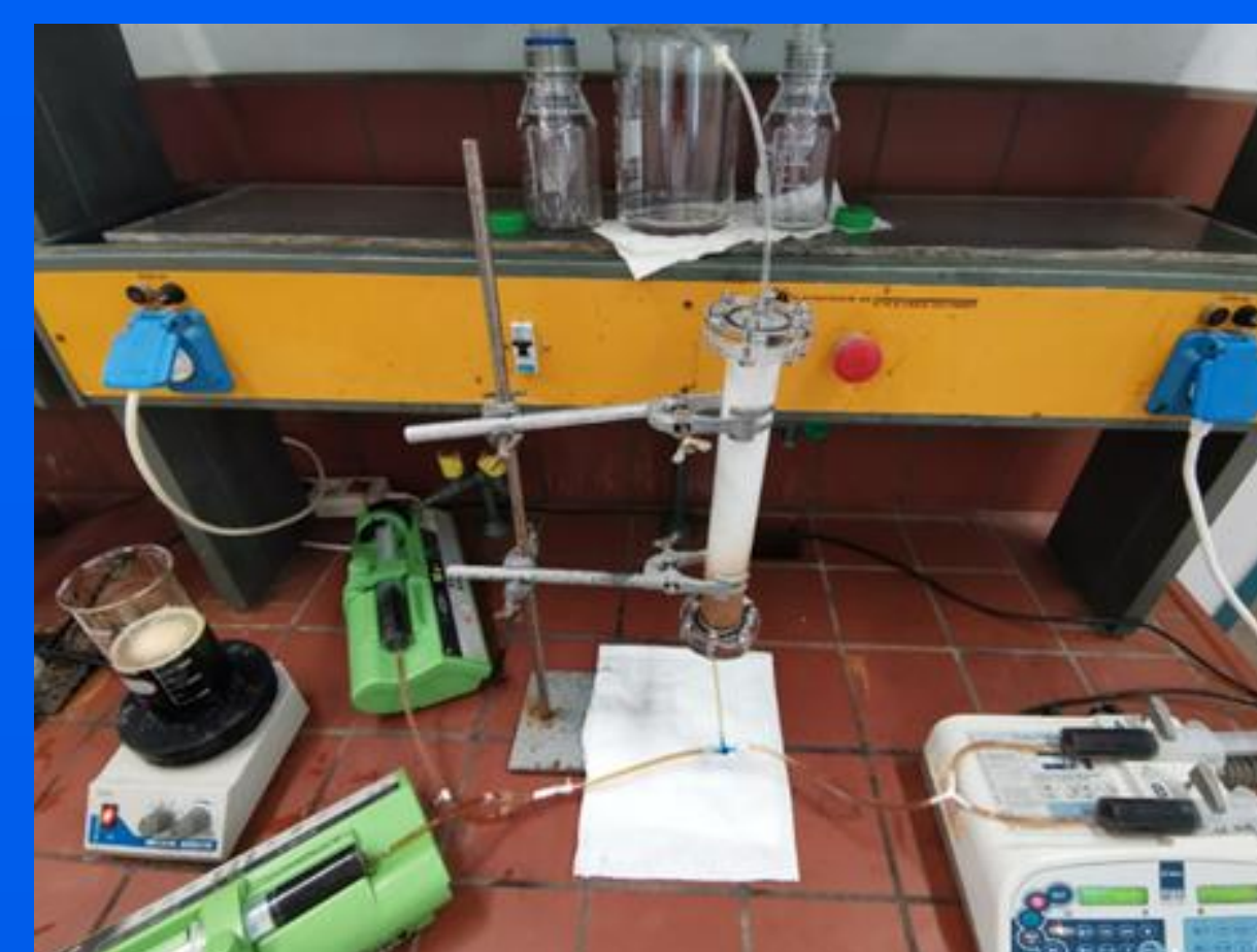
Figure 1: Experimental set-up for the adsorption/desorption processes. A 30-cm height column packed with XAD-16N resin (non-ionic, cross-linked polymer)
