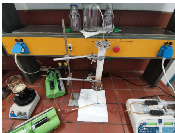
Figure 1: Experimental apparatus for the adsorption/desorption processes at constant flowrate of 300 ml/hr in a 30-cm height column packed with XAD -16N resin (non-ionic, cross-linked polymer)
