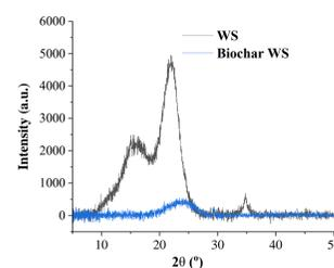
✓ There were three common peaks for raw WS at 2θ angles of 16.0°, 22.0° and 34.6° which are dependent on (110), (002) and (004) and all of them are related to cellulose type I. The broad peak in the XRD of raw WS sample and derived biochars at 2θ angle of 22.0° revealed the presence of an amorphous phase mainly consisting of cellulose, hemicelluloses, and lignin.
