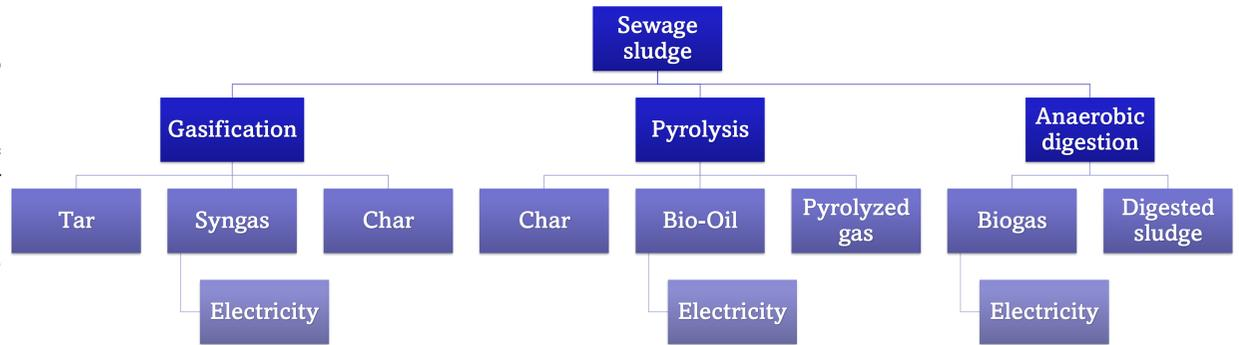
Figure 1: Routes of energy generation from sewage sludge
