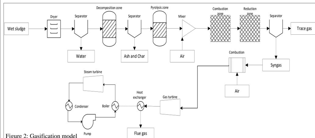
Figure 2: Gasification model
