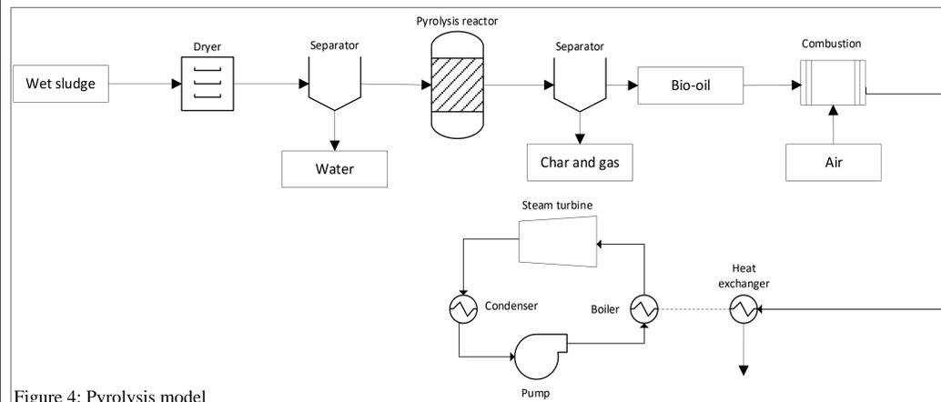
Figure 4: Pyrolysis model
