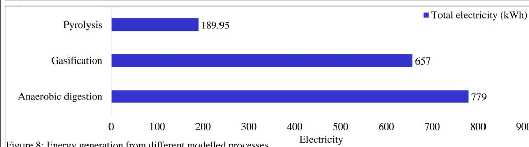
Figure 8: Energy generation from different modelled processes
