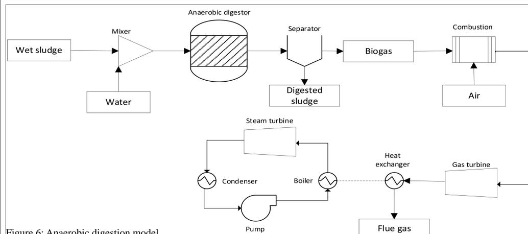
Figure 6: Anaerobic digestion model
