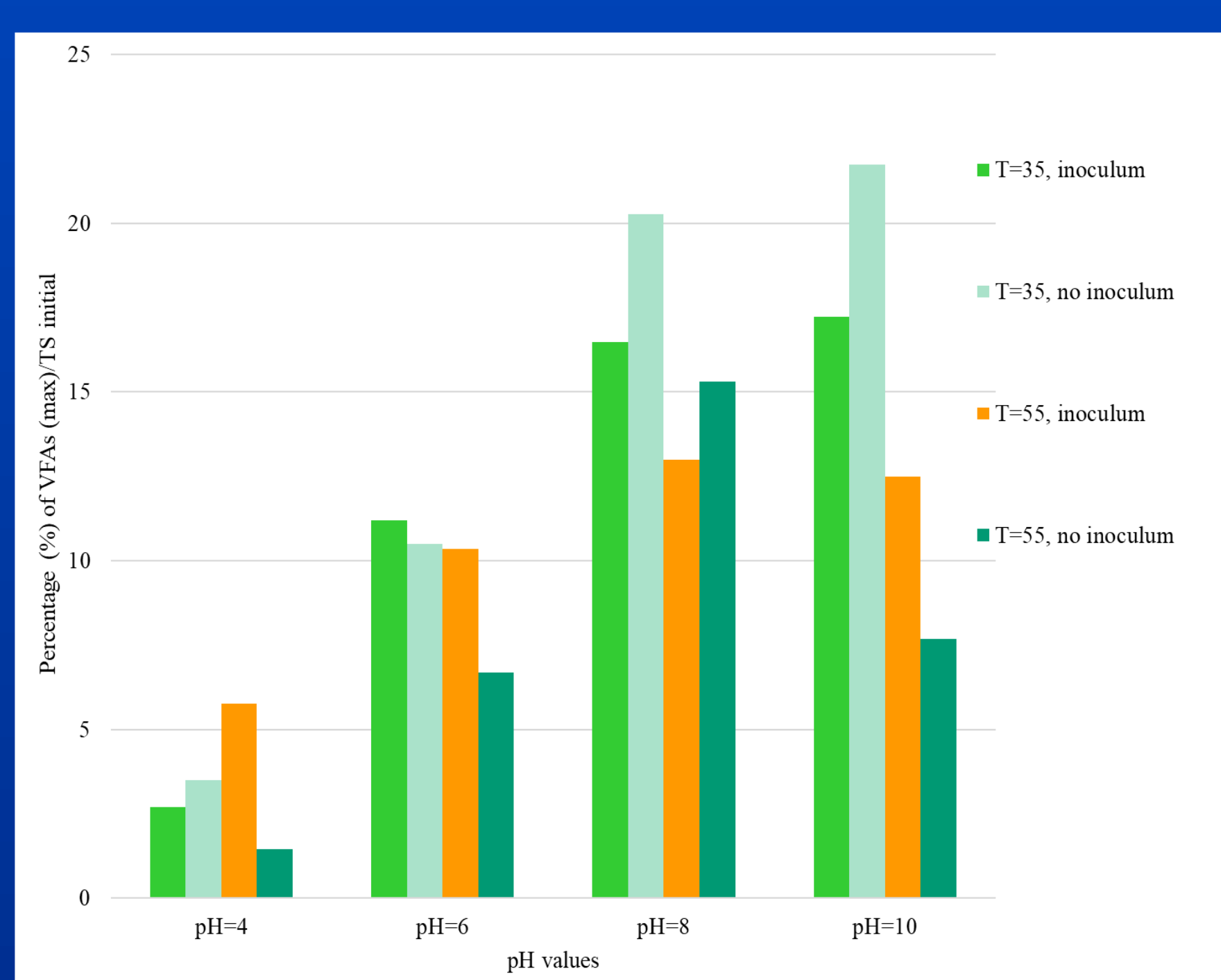
Figure 2: Maximum VFA production yields in FW fermentation, with and without the addition of anaerobic sludge, in mesophilic and thermophilic conditions
