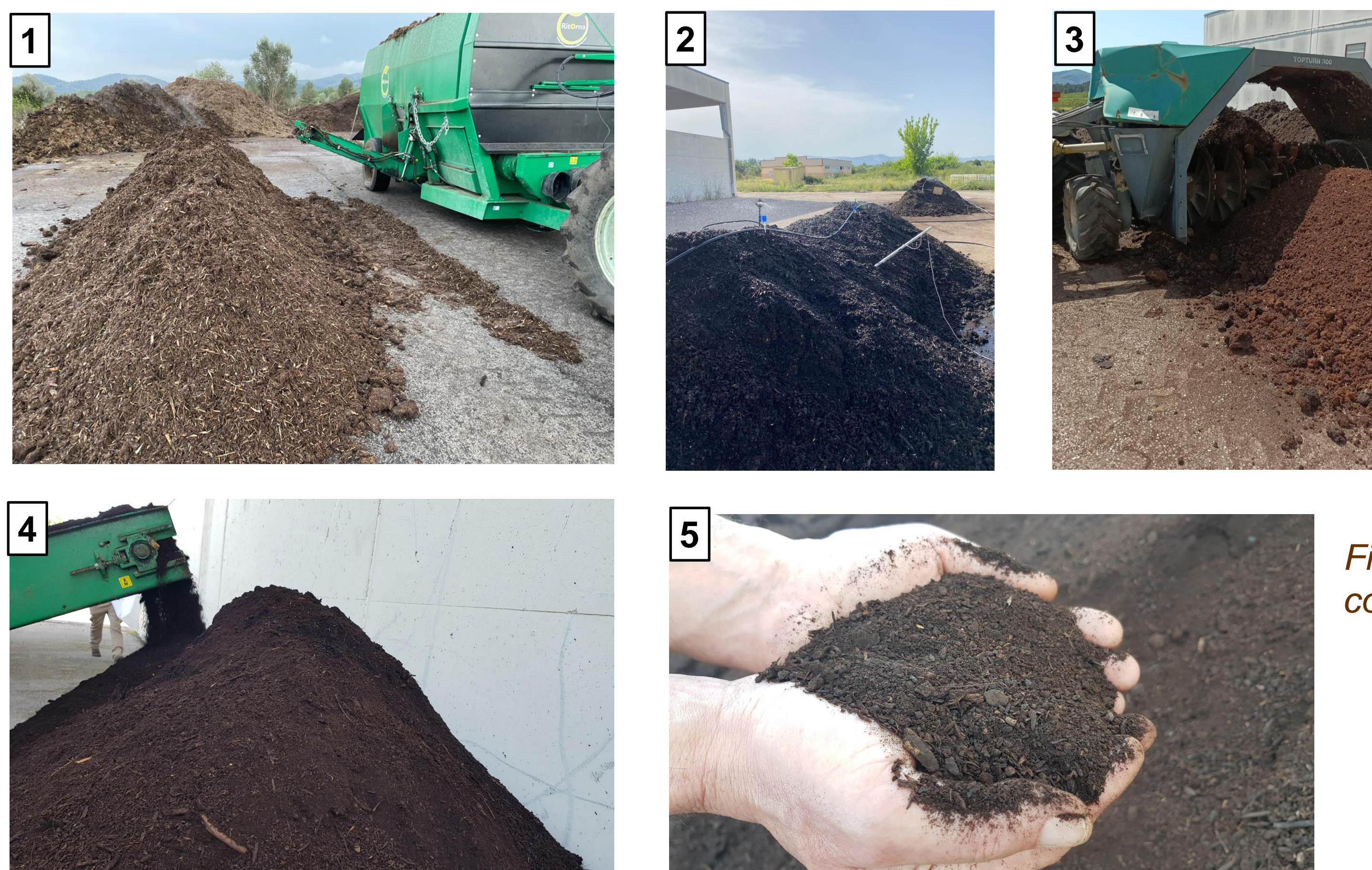
Figures 1, 2, 3: preparing start up mix, irrigation system, and turning.
