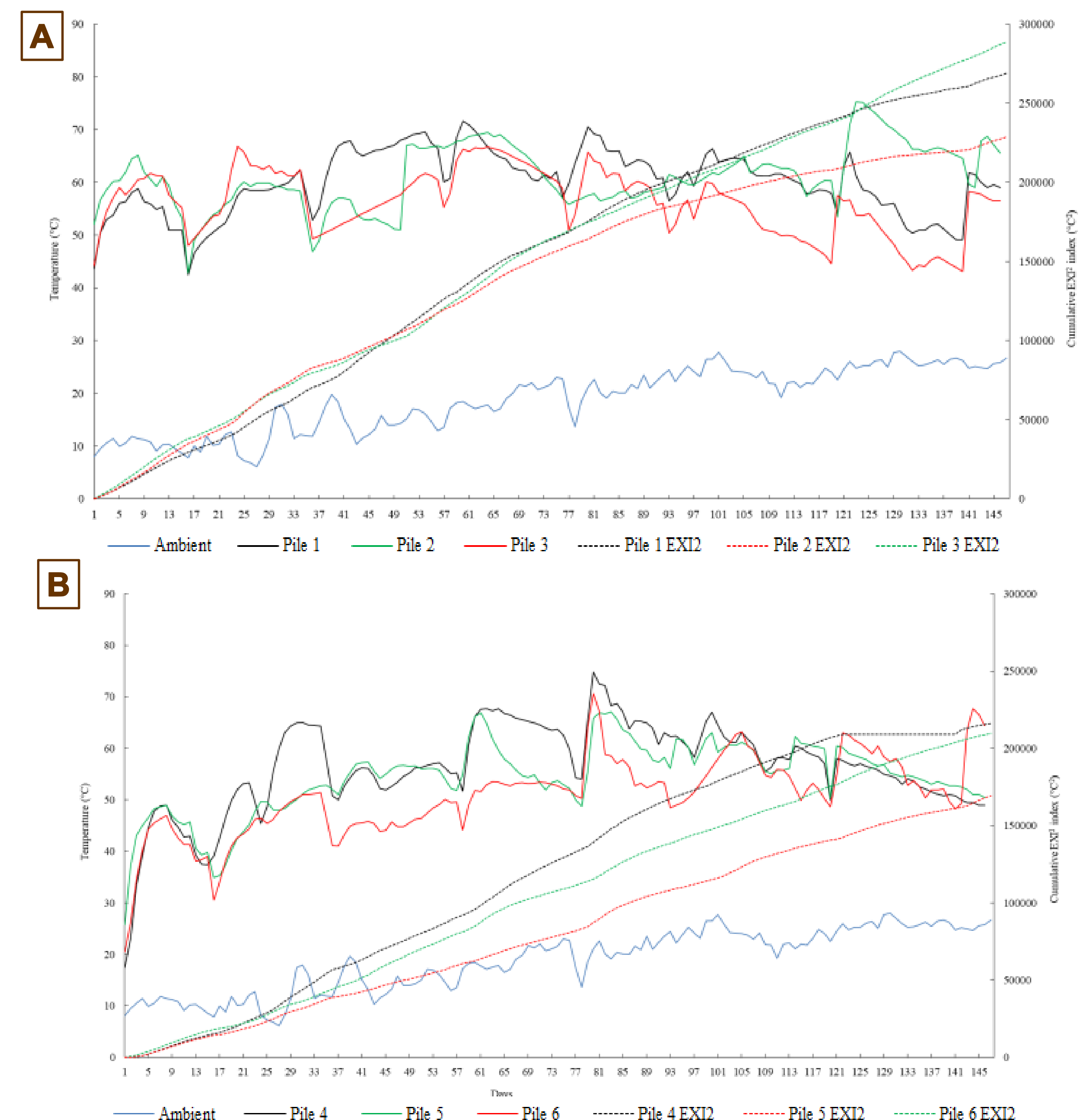
Figures 8 and 9. Evolution of the temperature and of the cumulative quadratic exothermic index (EXI2)
