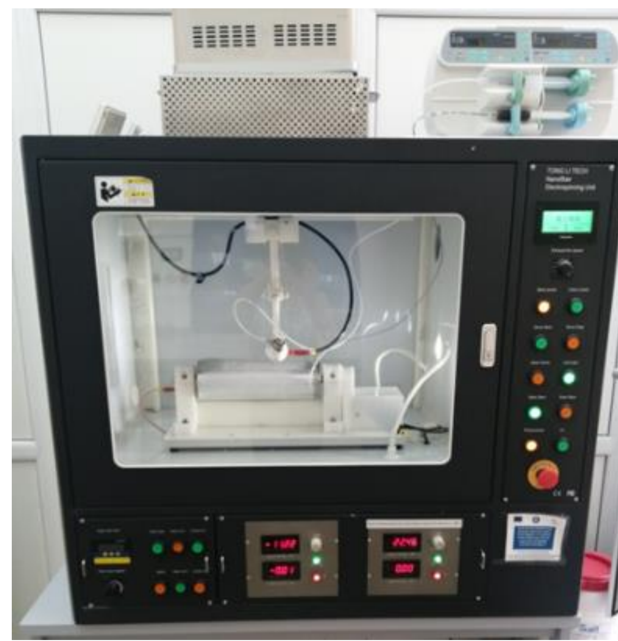
Figure 1: Mono- and coaxial electrospinning equipment used to obtain assembled PLA/PEO/Keratin-PVP/Collagen nanofibers
