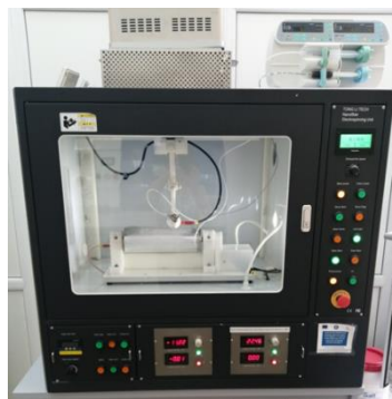
Figure 1 Mono- and coaxial electrospinning equipment used to obtain assembled PLA/PEO/KH/PVP/CH nanofibers.
