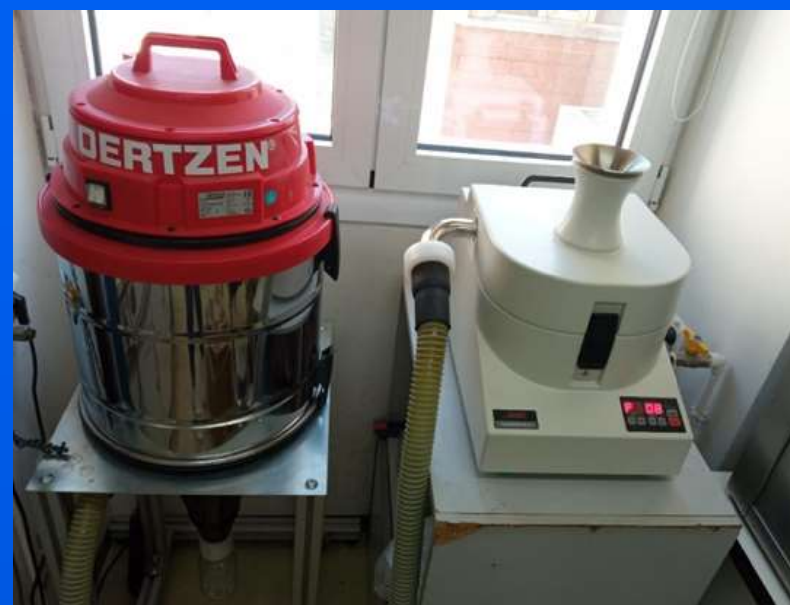
Figure 1: Cutting mill of WPPC
