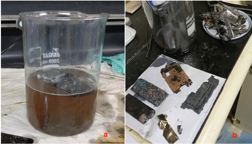
Fig 3. Batteries floating on the zinc chloride solution with density 1.8\text{ g.cm}^{-3} (a) and some tested components (b)
