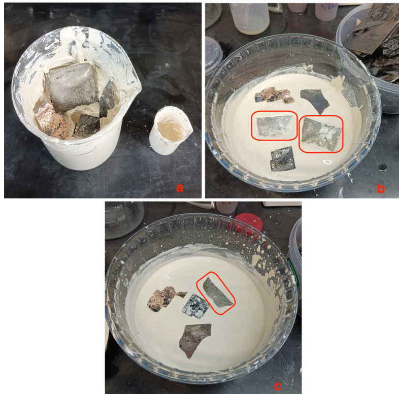
Fig 4. Pasty material of white-clay with density 1.8 \text{ g.cm}^{-3} and viscosity 35.7 \text{ g/(cm.s)} (a) Solution of viscosity 0.98 \text{ g/(cm.s)} and density 1.34 \text{ g.cm}^{-3} with batteries into red squares (b). Solution of viscosity 0.2 \text{ g/(cm.s)} and density 1.28 \text{ g.cm}^{-3} with a battery into a red square (c).
