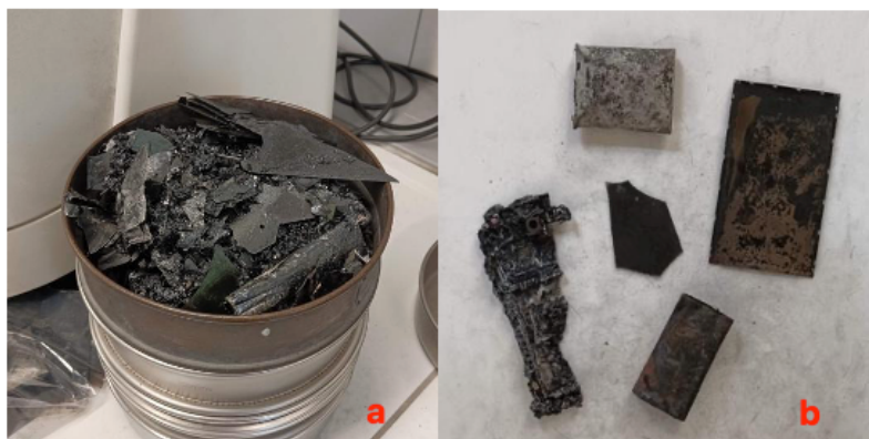
Fig 1. Mobile phone components after pyrolysis (a) and after 2 cm sieving (b)
