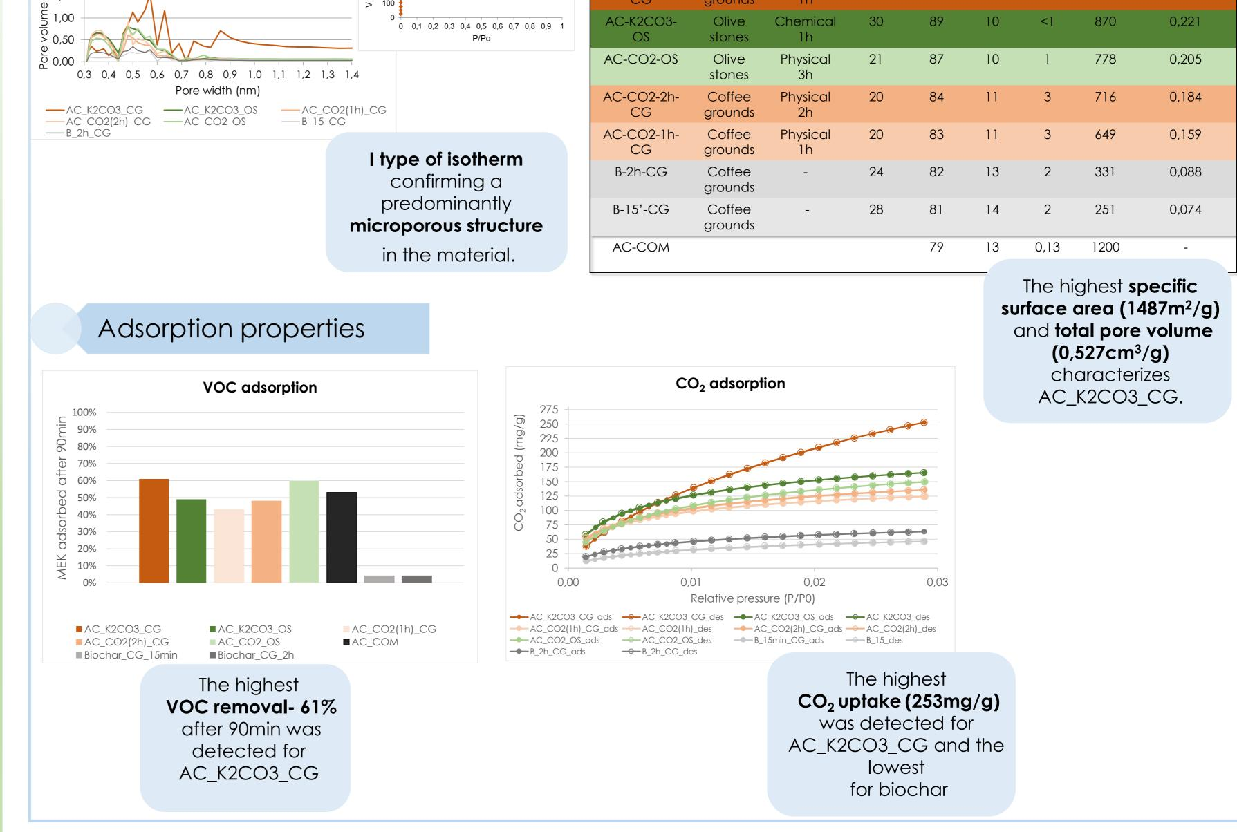
Measurements of VOC adsorption were performed in a 17L chamber, at room temperature where 50mg of each sample was placed and Methyl Ethyl Ketone (MEK) was chosen as a model of VOC. The concentration was monitored for 90min using a photoionization detector (PID).
