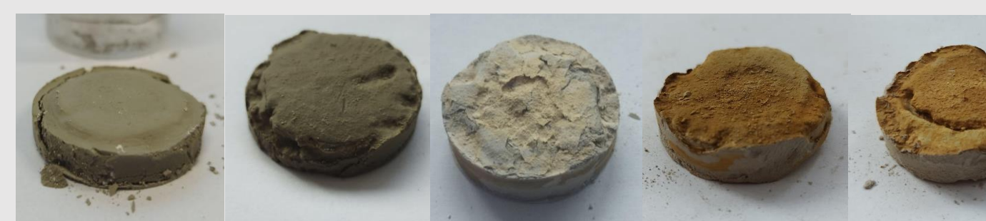
WCF – highway: Composites prepared for testing mechanical properties (the testing is still in progress).
