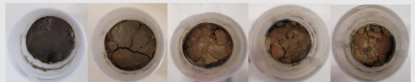
WCF – gutter: Composites after 7, 14, 30, 60 and 90 days
