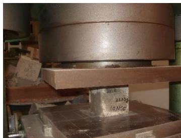
Fig.1. Determination of compressive strength in the laboratory
