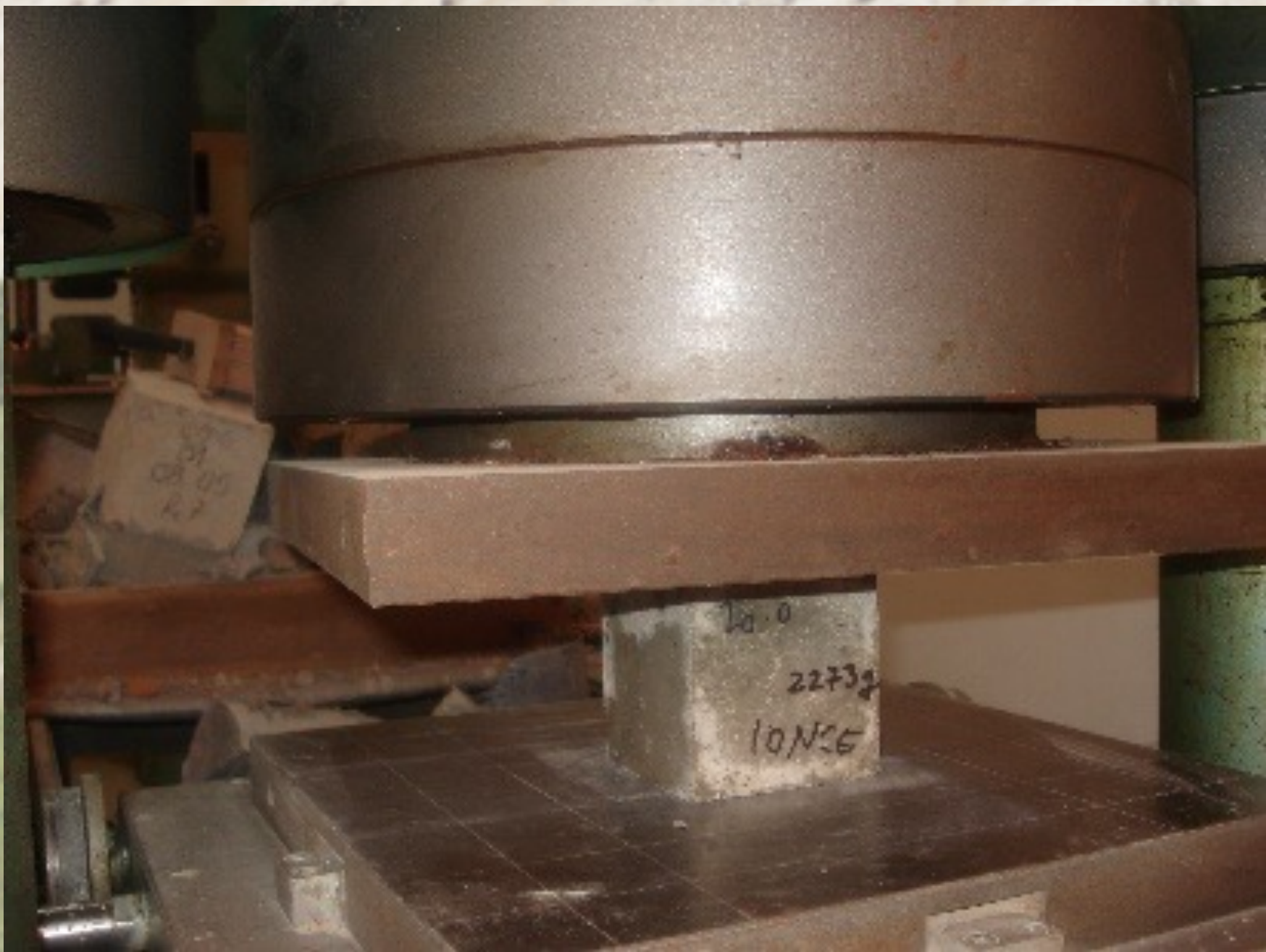
Figure 2: Determination of compressive strength in the laboratory
