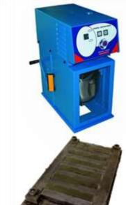
**Precursor addition** and planetary mixer homogenization (120 s)
