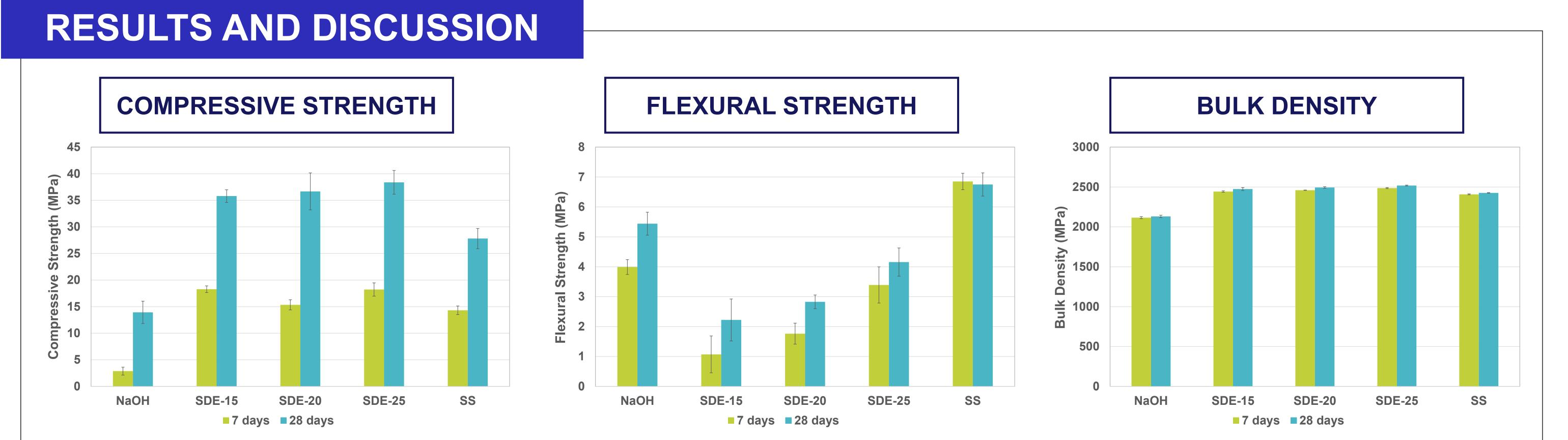
Results showed that materials activated with spent diatomaceous earth reached higher compressive strength and similar bulk density than those activated with commercial sodium silicate. Best results were obtained by specimens with 25g of spent diatomaceous earth for every 100 ml of sodium hydroxide solution.
