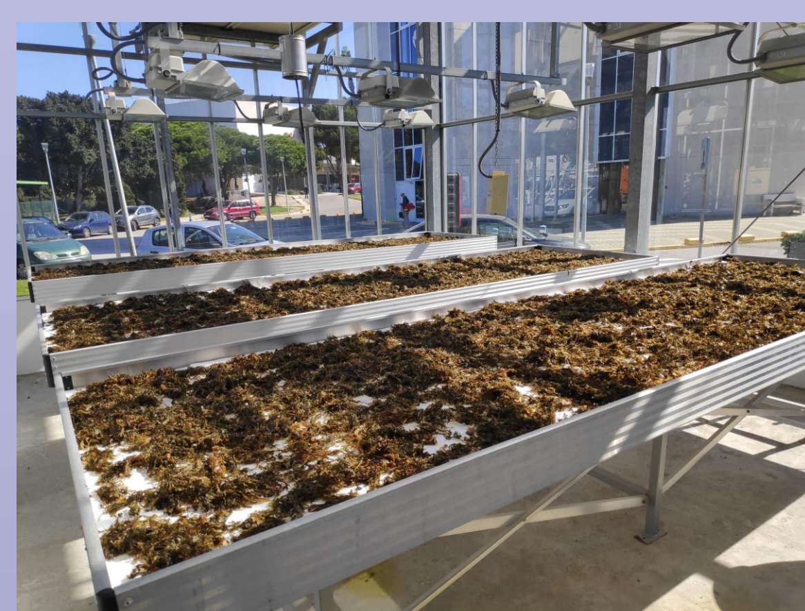
Figure 1. Conditioning macroalgae: above: washing system; below: drying system
