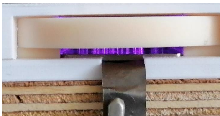
Fig. 1: Atmospheric plasma reactor for polymer foils treatment
