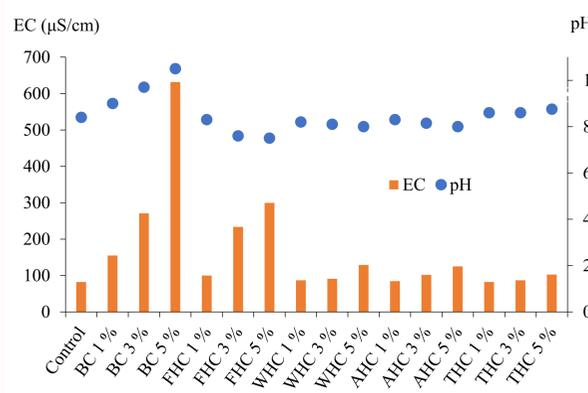
Fig. 2. pH and EC of stabilized soils
