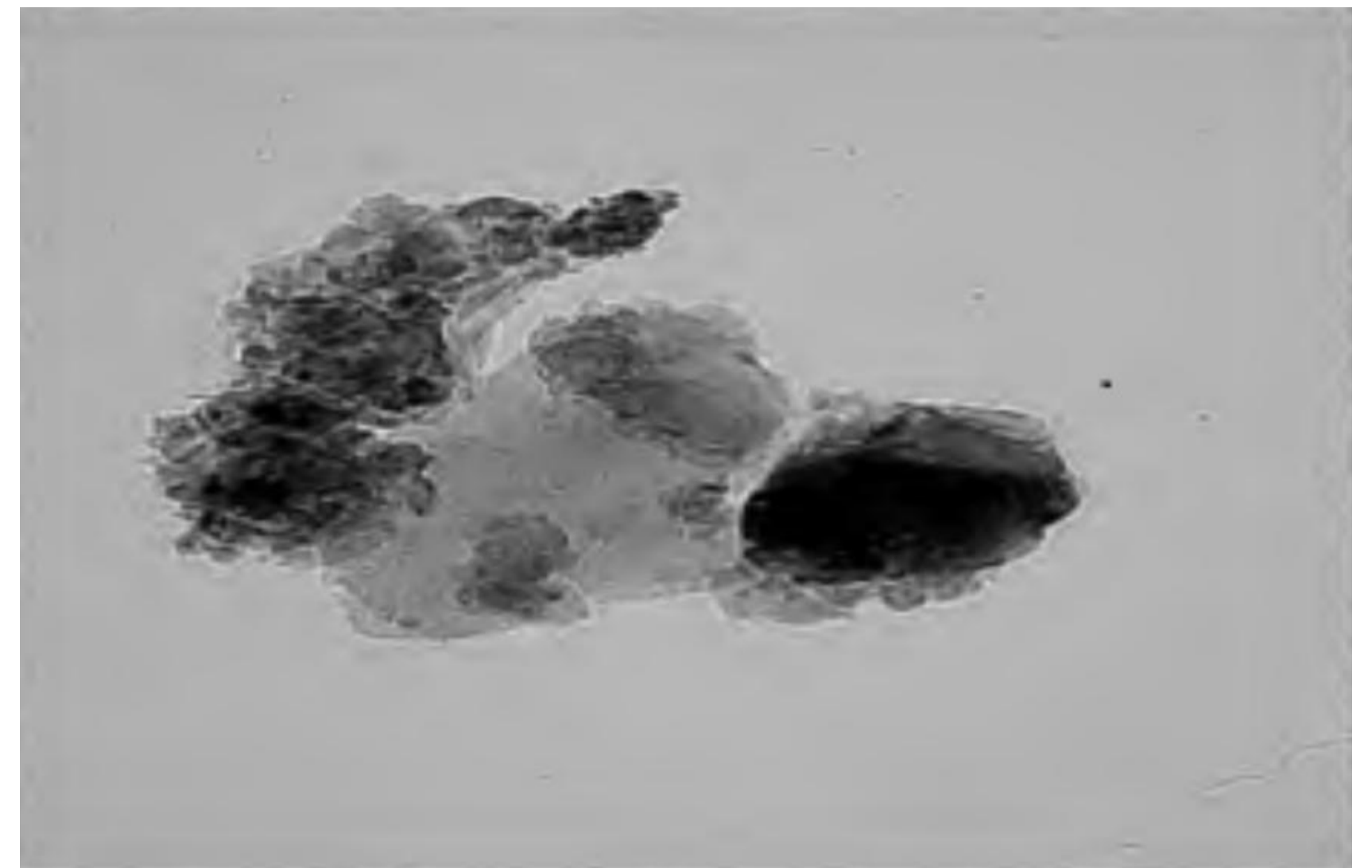
Figure 2. Powder of metallurgical industry technogenic waste after grinding on the planetary mill and further centrifugation
