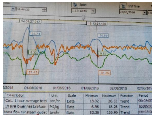
Figure 5D DCS extracted graph indicating the correlation between Calorific Value the orange line, waste throughput the blue line and HP steam production the green line
