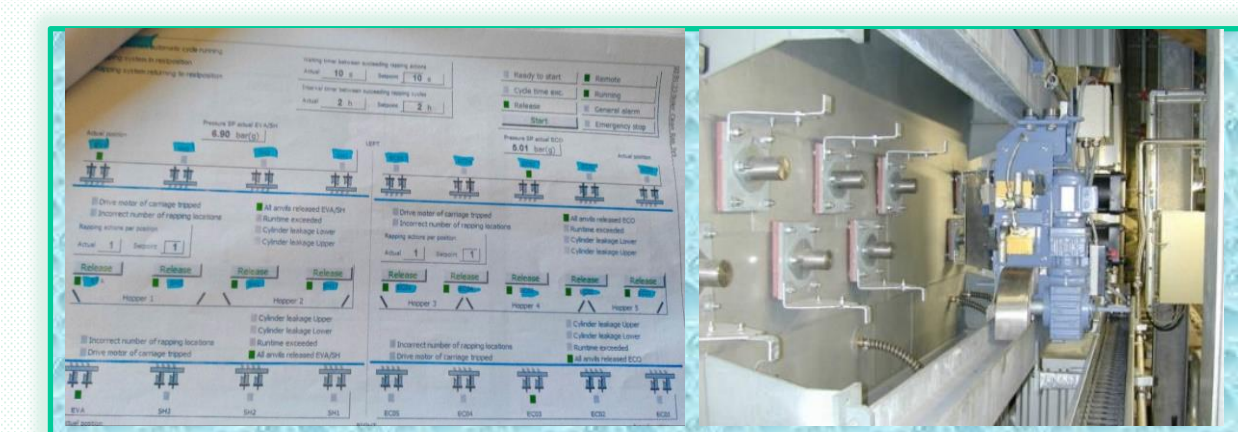
Figure 7 The boiler rapping system
