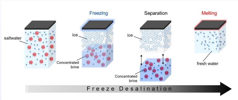
Figure: Freeze desalination process
