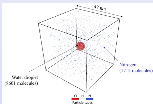
Figure: Initial state- equilibrated at 1 bar 273K
