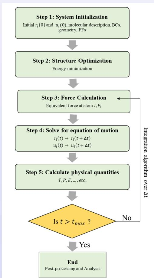
Figure: Molecular dynamics flow chart
